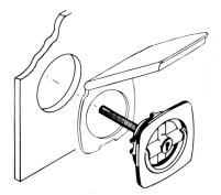
Typical installation and positioning on Cat. Nos. 1031/1032 Series Lock/Latch Sets.
