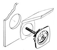
Typical installation and positioning on Cat. Nos. 0931/0932 Series Lock/Latch Sets.
